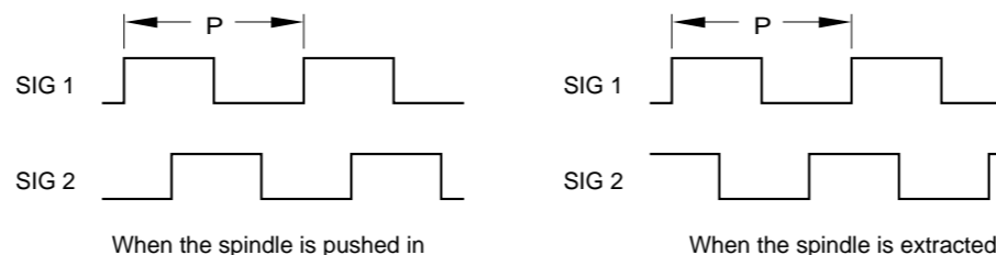
*1: GS-1500A Series: 68 \Omega , GS-1630A: 220 \Omega P = 40 \mu m or 4 \mu m
